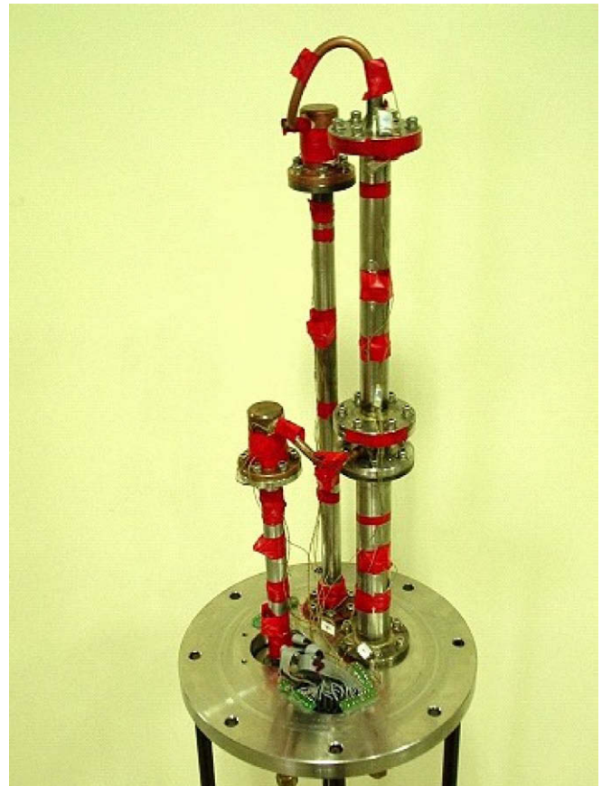
Fig. 2. Photograph of the two-stage Pulse tube system.
